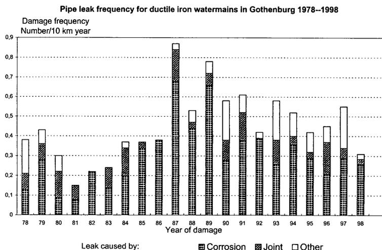
**Figure 4** Damage frequency of ductile-iron water pipelines in Gothenburg during the period 1978 – 1998. First year of burial of ductile- iron pipes: 1969 (Data from O. Ljunggren, Gothenburg Waterworks, personal communication, 2000)
