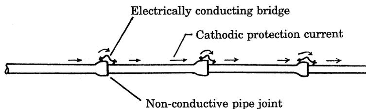
Figure 1 Electrically conductive bridging of non-conductive pipe joints (Camitz 1995)
