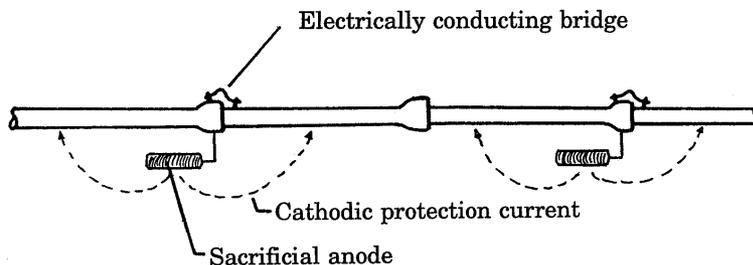
**Figure 3** Cathodic protection with sacrificial anodes of ductile-iron water pipes with non-conductive pipe joints. Each anode protects two pipes, and consequently only every second pipe joint has to be bridged (Camitz 1995)
