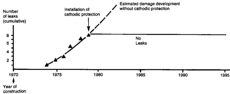
**Figure 2** Corrosion damage development (water leaks) on a steel water main (DN 400) outside Stockholm, and the protective effect of a cathodic protection installation during 17 years (Camitz 1995)
