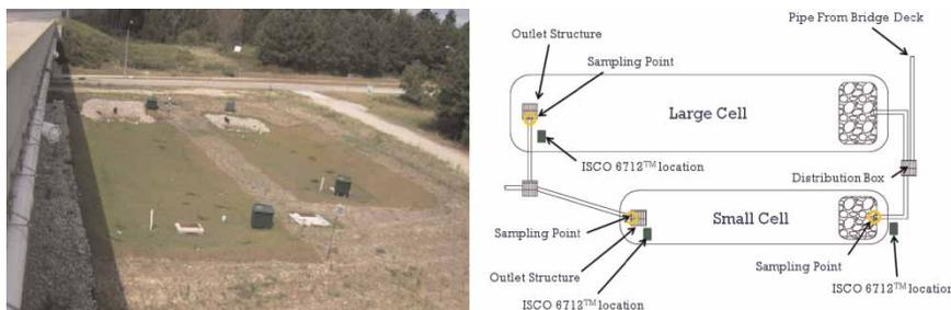
**Figure 1** | (a) Standard (left) and undersized (right) bioretention cells at Mango Creek (left image). (b) Bioretention cells schematic (right image).
