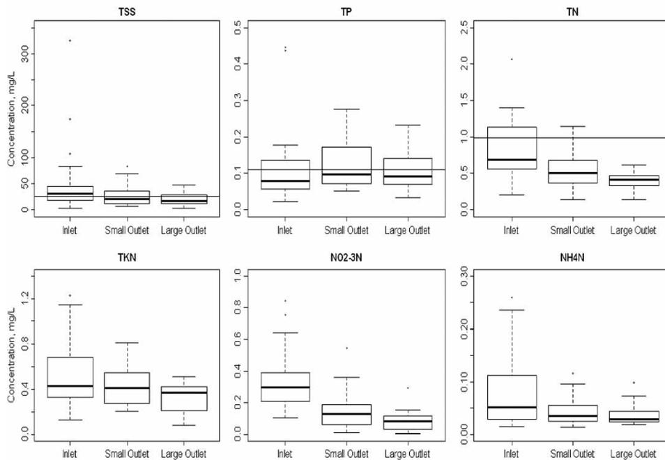
**Figure 2** | Box plots of nutrient and TSS concentrations ( $n = 24$  inlet to large cell outlet,  $n = 29$  inlet to small cell outlet, and  $n = 23$  large cell outlet to small cell outlet). Horizontal lines represent target North Carolina water quality standards in the Piedmont region for TSS, TP, and TN.
