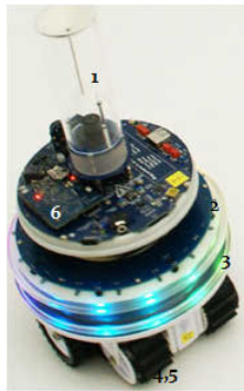
Figure 1: A footbot. Sensors and actuators are placed as follows: (1) omni-directional sensing camera, (2) proximity sensors, (3) LEDs, (4,5) wheels and ground sensors, (6) RAB sensor and actuator
