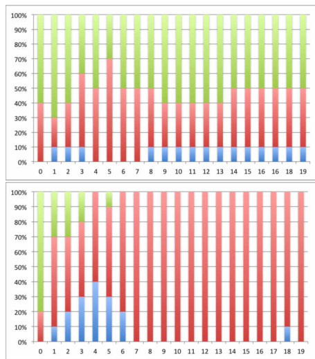
Figure 10: Distribution of coordination patterns amongst robots in each time interval. The top figure shows Arena 1, the lower Arena 3. The figures are 'stacked' in the order blind diffusion, RACO, AMORPH from the bottom
