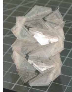
Fig. 4. Self-folded structure, which consists of 62 mountain and valley folds.
