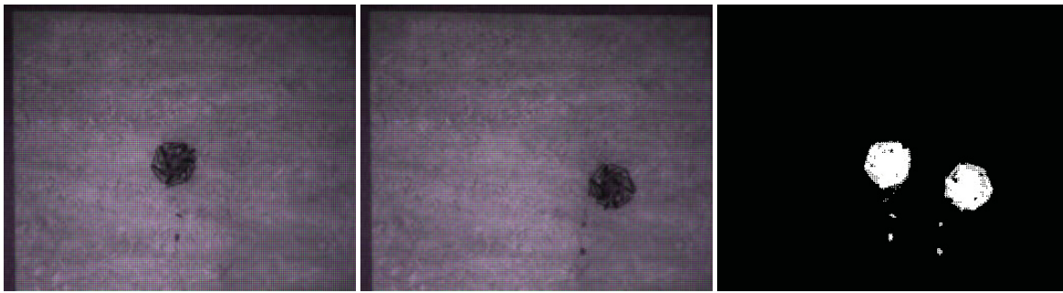
Figure 6: An example of how distance traveled was automatically measured. Position was calculated by subtracting an “empty” arena image from one containing the robot. Distance could then be measured by comparing beginning (left) and final (center) robot positions (right).
