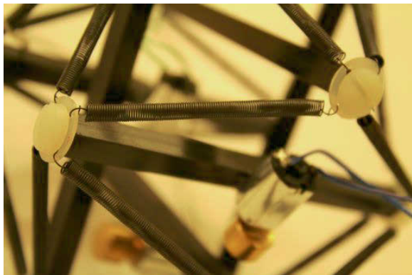
Figure 3: The body of the tensegrity robot consists of rigid plastic rods and metal springs. It is actuated by simple DC vibrating motors attached at the midpoint of three of its six struts. A closeup of the robot illustrated the springs and the DC motors. (Photo by Steven Stangle)
