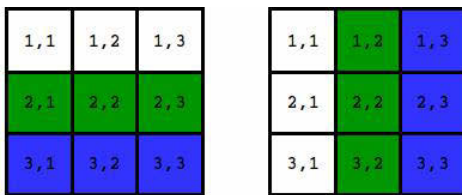
Figure 2: This illustrates the naive coordinatization of the 3 \times 3 world. We show the world grid and overlay the coordinatization, the tuples in each grid position denote f_{(A,B)}(x) = (f_A(x), f_B(x)) where x is the state label fixed to the grid position as described in the text. The left (right) diagram highlights the partition A ( B ) with each block a ( b ) given the same color.
