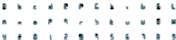
Figure 3: “All characters and numbers printed by self-assembly printer”.
