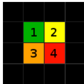
Figure 13: A 2x2 Positional Metacell. Each interior cell is encoded by its position within the metacell.
