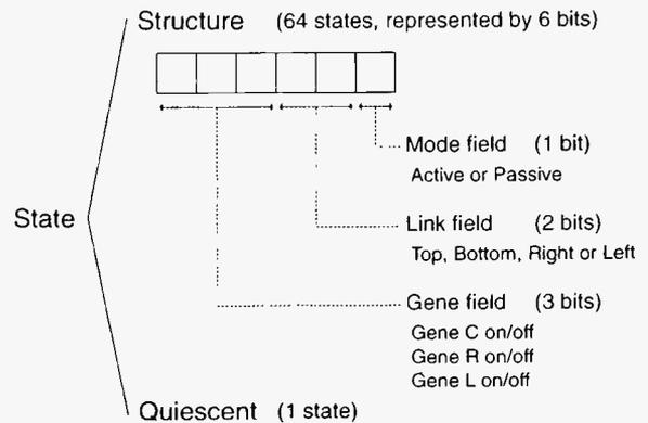
Figure 3: Design of states in the new model.
