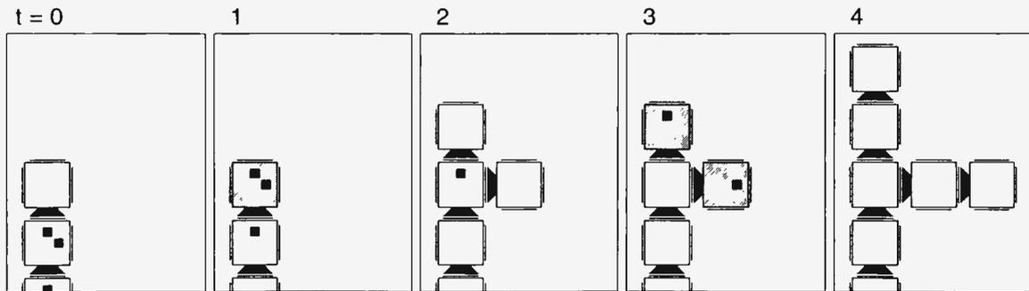
Figure 5: Shape decoding process at the head of a pattern. The uppermost cell to which no cell is rooted becomes active at the arrival of genes ( $t = 1$ ). This active cell stimulates its adjacent quiescent sites to let them turn into blank structure cells according to direction by the genes ( $t = 2$ ). Such a process takes place repeatedly ( $t = 3, 4$ ).
