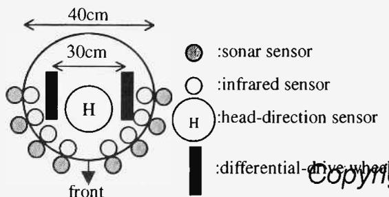
Figure 2: Sensors and actuators of the animat
