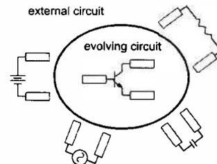
Figure 8: By associating sequences of characters to the terminals of the external devices, connections from the circuit specified by the genome (shaded region) to the external devices can be subjected to evolution.
