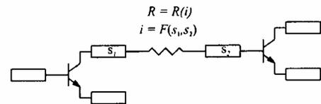
Figure 4: The strength of the connection between devices can be assigned by associating sequences of characters to the terminals, defining a mapping  $i = F(s_1, s_2)$  from pairs of sequences to values of connection strength, and a further mapping  $R(i)$  that gives the values of resistance.
