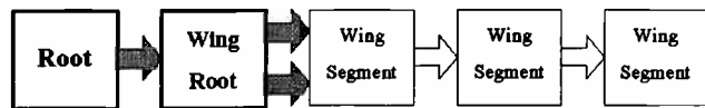
Figure 2: A genotype structure. The wing-root has double connections for two symmetric wings.
