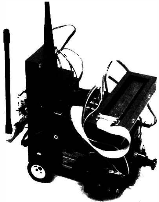
Figure 2: The robot used, 16cm×12cm×15cm excluding aerials, weighing 800g and supported by two independently driven wheels and a coaster attached front centre. The maximum speed used for this experiment was 2.5cms -1 .
