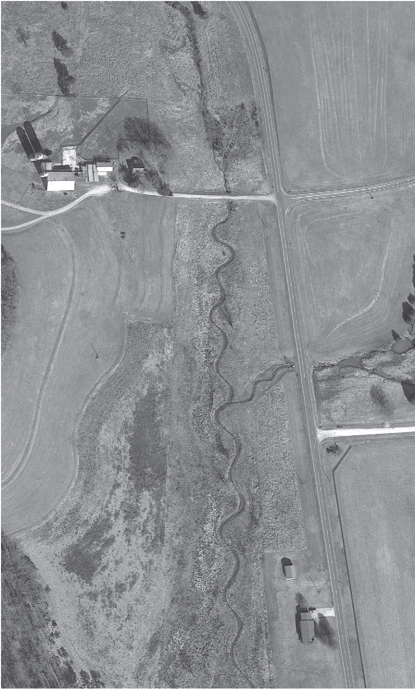
Figure 1.1 Aerial image of Martin Dairy Creek, North Carolina. The stream flows from top to bottom, with the portion upstream of the farm road being unrestored—and perfectly straight—while the downstream portion is restored into almost perfectly symmetrical sine wave meander bends.
