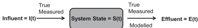
Figure 3.1 Influent, effluent and system state as functions of time. The effluent can be modelled using the measured influent and a model representation of the system state.
