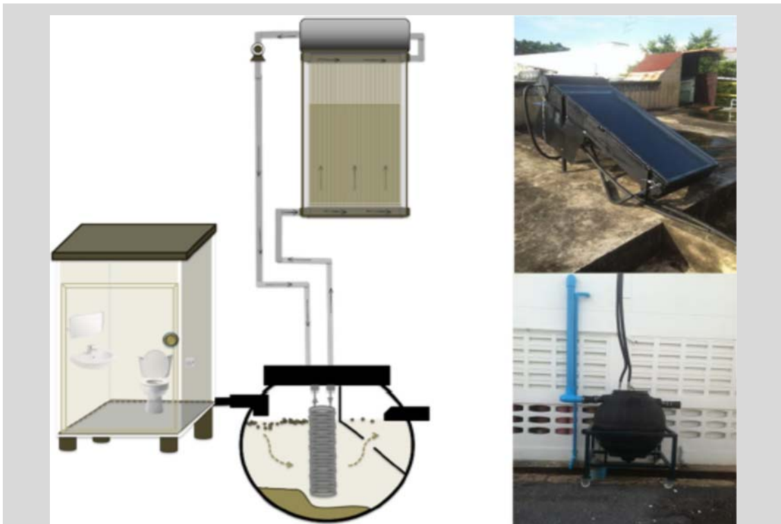
Figure 3.3 Field testing of the solar septic tank at the Asian Institute of Technology, Thailand (Source: AIT 2015).
