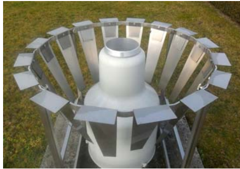
Figure 2.5 Rain gauge with fence against wind effects. Source: Patrick Willems (KU Leuven).
