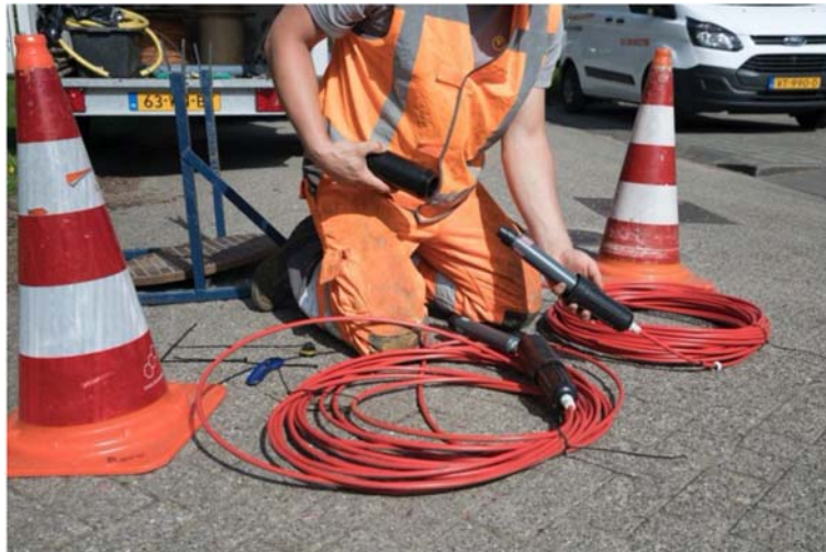
Figure 6.15 Connecting cable segments using an optical connector for DTS measurements. Source: courtesy Remy Schilperoort (Partners4UrbanWater).
