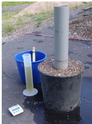
Figure 5.3 Items required for the field test of the infiltration capacity of filter material for VF wetlands according to EN 12566-2 (2005).
