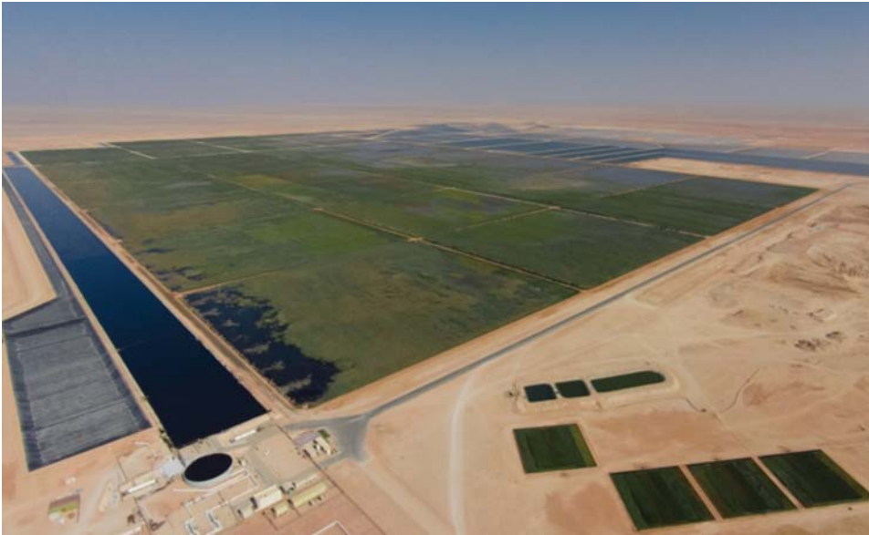
Figure 40.1 Aerial view of the Constructed Wetland facility for oily produced water treatment in Oman. (Courtesy: Bauer Nimr LLC)
