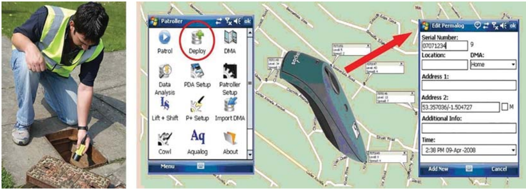
Figure 6.5 Lift and shift deployment and GPS mapping function. (Source: Halma Water Management)
