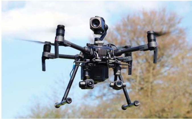
Figure 10.3 A drone equipped with cameras for leak surveys. (Source: Bath Echo)
