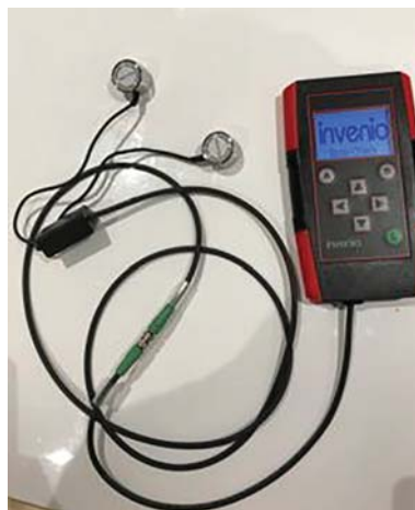
Figure 16.3 Vibration recorder. (Source: Invenio Systems)
