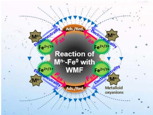
Figure 5.4 Proposed schematic illustration of the reactions of ZVI with Se(IV)/Se(VI) in the presence of a WMF (Li et al. , 2020a).
