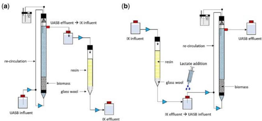
**Figure 7.7** Schematic of the integrated treatment system comprising of an IX column and a UASB reactor. The process flow configuration was evaluated as either (a) IX as post treatment of the UASB or (b) IX as pre-treatment of the UASB influent (Cáliz *et al.*, 2019).
