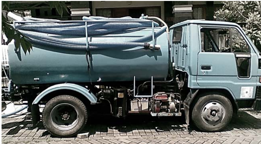
Figure 10.2 The most important parts of a desludging unit are (1) sludge tank, (2) vacuum pump, and (3) desludging hose. Each unit must also carry safety equipment and first-aid kit box.
