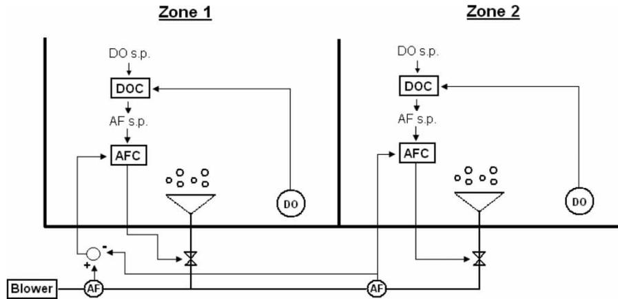
**Figure 3** | Visualisation of the overall control of the test line. DOC is the DO PI-controller and AFC is the airflow PI-controller. The circles with DO and AF represent online measurements of DO and airflow (modified from Larsson 2011).
