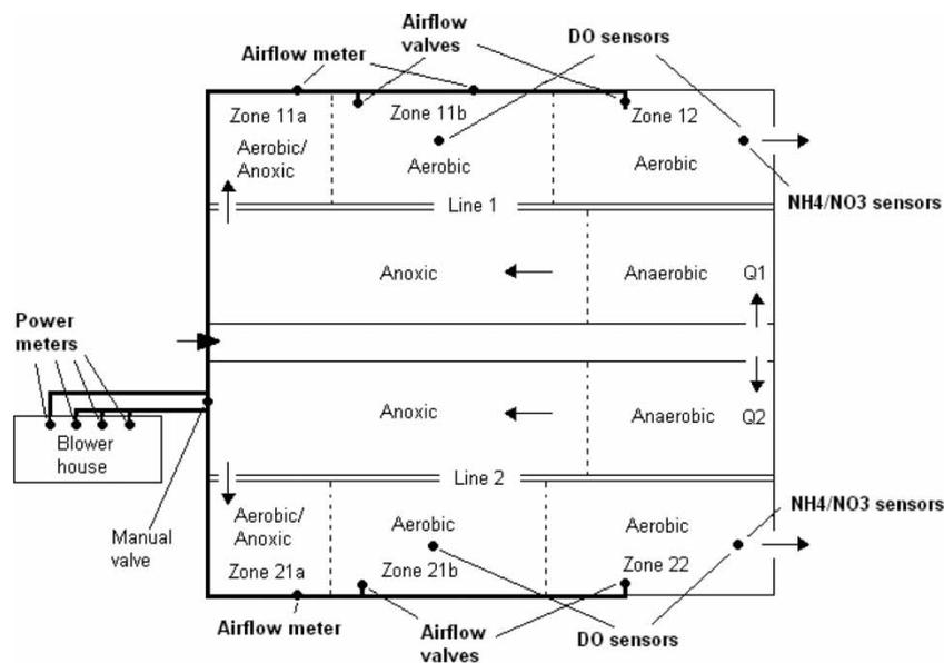
**Figure 2** | Position of on-line measurements in the biological treatment step at the test plant (Larsson 2011).
