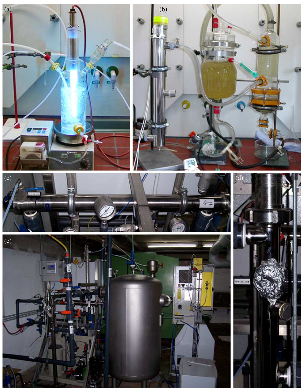
Figure 1 | Photographs of the four different reactors for UV treatment in combination with H_2O_2 . (a) laboratory reactor equipped with a Hg-LP-lamp, (b) semiworks equipped with a Hg-LP-lamp, (c) Hg-LP-lamp and (d) Hg-MP-lamp of the (e) pilot plant.
