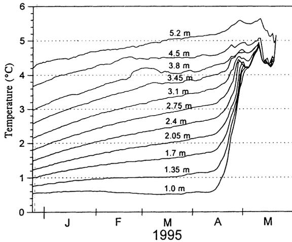
Fig. 5. Thermistor chain recordings in a vertical in the deep part of Lake Uros during the period December 25, 1994, to May 25, 1995. The ice break-up occurred about May 20. The bottom depth is 5.5 m.
