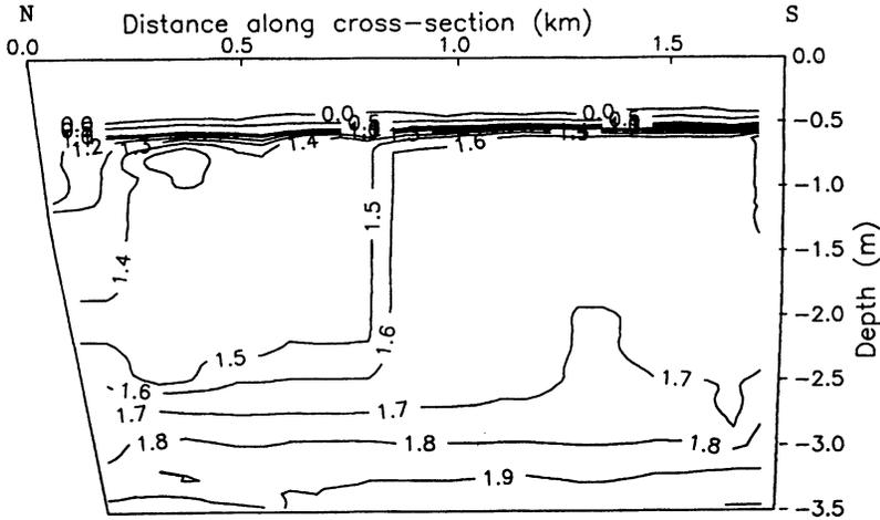
Fig. 17. Temperature distribution in the upper 3.5 m layer along cross-section 4 in Lake Vendurskoe during the evening of April 22. The isotherm spacing is 0.5°C between 0°C and 1°C, and 0.1°C between 1°C and 2°C. Left-hand side of the figure corresponds to the northern part of the section, and the right-hand side the southern part.
