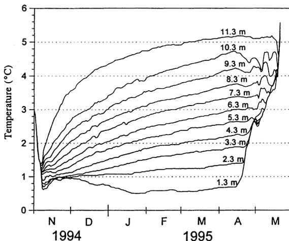
Fig. 3. Thermistor chain recordings in a vertical in the deep part of Lake Vendyurskoe during the period October 24, 1994, to May 24, 1995. The ice formed on November 8, and broke about May 20. The bottom depth is 11.3 m.
