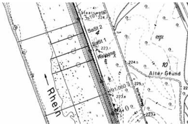
Figure 6 | Field site with sampling stations (SaSt1, SaSt2), release station and surveyed cross sections 191.06 km and 191.29 km marked.
