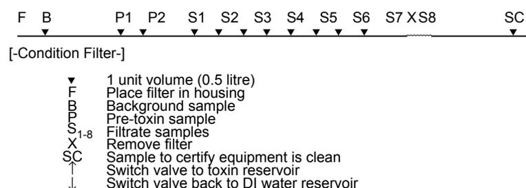
**Figure 1** | Diagrammatic representation of the sampling protocol.
