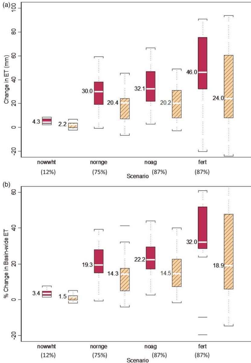
**Figure 7** | Differences in basin-wide (a) spring (solid) and summer (striped) eT associated with switchgrass production and (b) the percent change in spring and summer eT relative to baseline in all scenarios during the simulation period, 1995–2009. The boxplots are read as for Figure 5.
