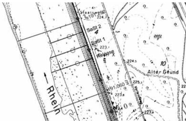
**Figure 6** | Field site with sampling stations (SaSt1, SaSt2), release station and surveyed cross sections 191.06 km and 191.29 km marked.
