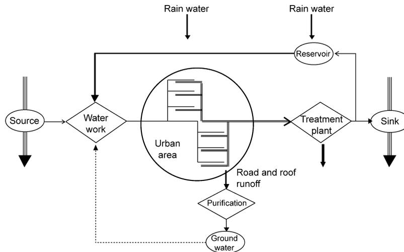
**Figure 4** Direct water re-use, taking water reservoirs and groundwater as close-to-nature holding facilities, and as means to enhance acceptability of the re-used water by the customers
