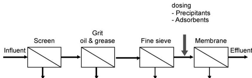
**Figure 5** Schematic of an advanced physico-chemical treatment train
