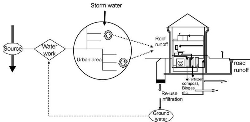
**Figure 2** Schematic representation of a “decentralized” system where the wastewater is treated close to the point of origin
