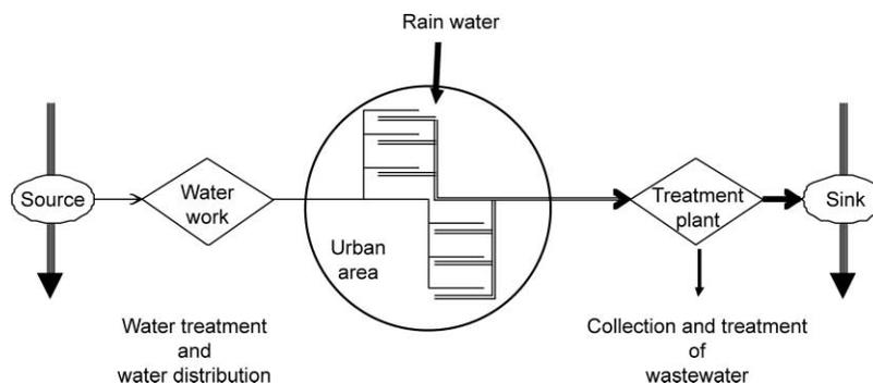
**Figure 1** Schematic representation of a “central” water/wastewater management system
