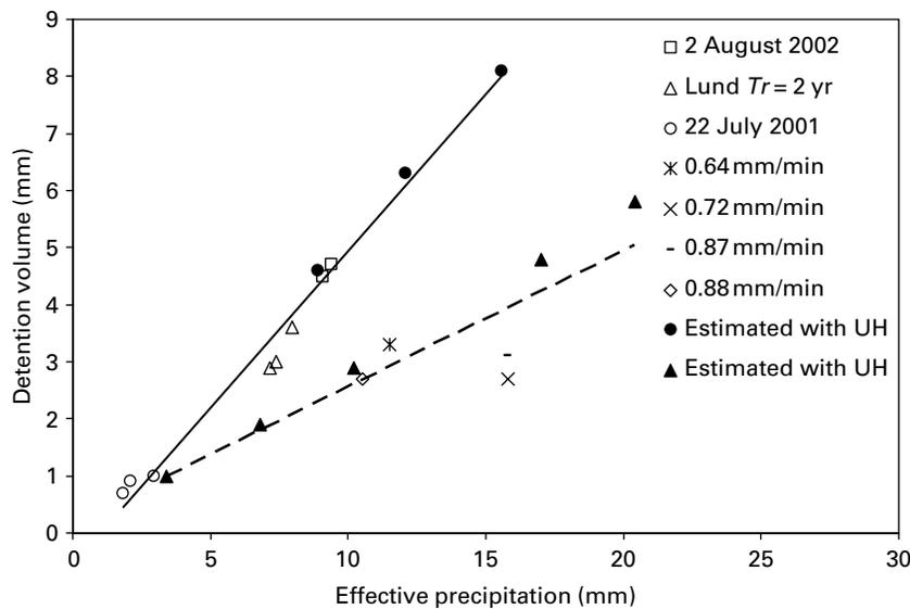
**Figure 4** Relationship between effective precipitation and detention volume. Continuous line shows the trend for events with variable rain intensity; dashed line shows the tendency for events with constant rain intensity
