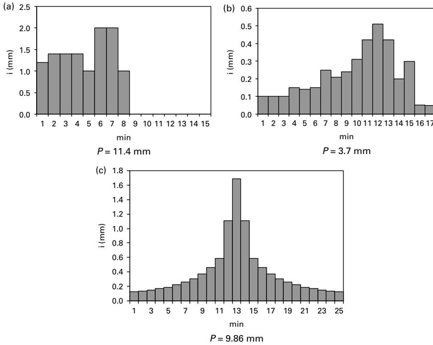
**Figure 1** Storm events used for the experiments: (a) 2 August 2002, Malmö; (b) 22 July 2001, Malmö; (c)  $T_r = 2$  yr for Lund.  $P$  indicates the total amount of precipitation
