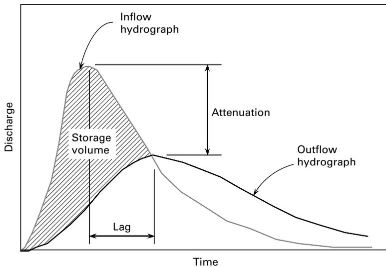
**Figure 2** Inflow and outflow hydrographs for a detention facility
