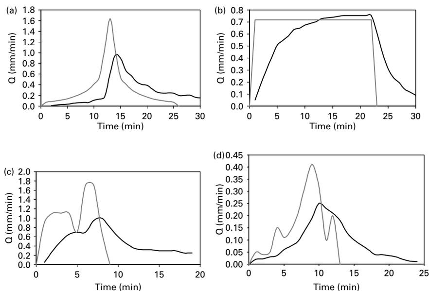
**Figure 3** Hard roof "inflow" (grey line) and green-roof "outflow" (black line) hydrographs for (a) Lund  $Tr = 2$  yr, (b)  $0.8$  mm/min, (c) 2 August 2002, (d) 22 July 2001
