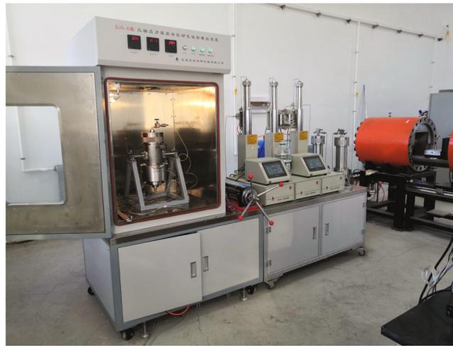
FIGURE 2: Photo of the triaxial stress coal-rock seepage experimental apparatus.
