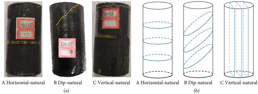
FIGURE 1: Prepared coal samples with different beddings. (a) Photo of the prepared coal sample. (b) Sketch of the bedding direction in the fractured coal.
