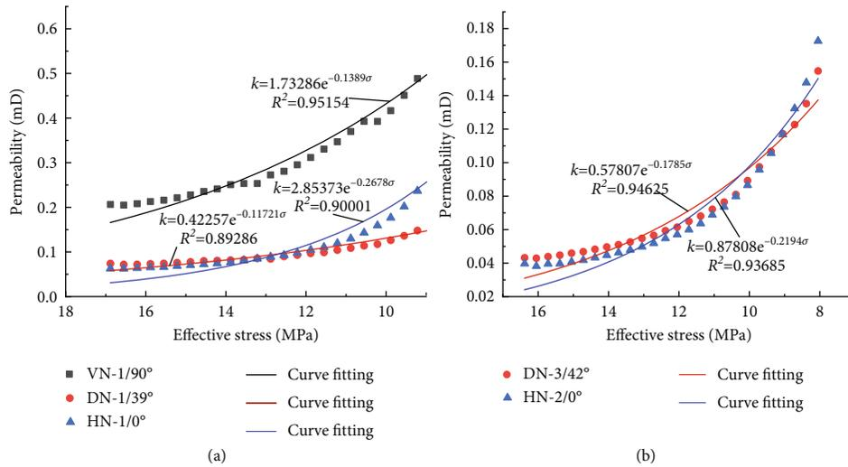
FIGURE 7: Permeability change of different bedding coal samples during stress unloading. (a) Gas pressure of 1 MPa. (b) Gas pressure of 2 MPa.
