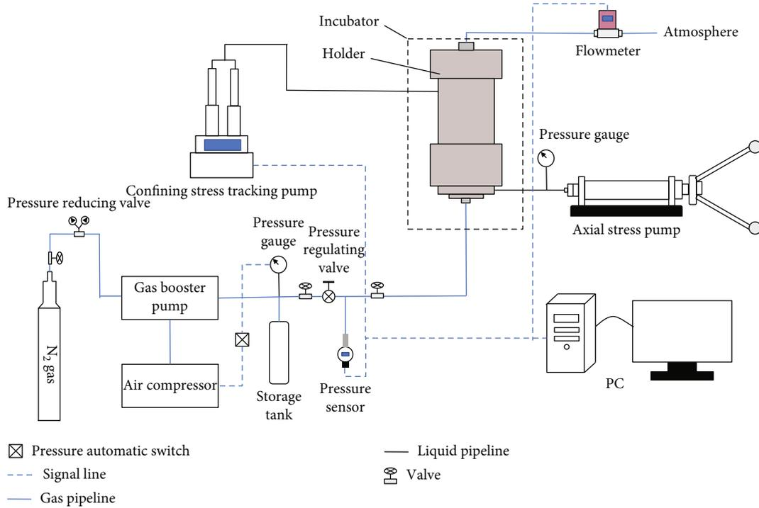
FIGURE 3: Principle of the triaxial stress coal-rock seepage experimental apparatus.
