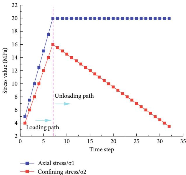
FIGURE 4: Stress loading and unloading scheme.
