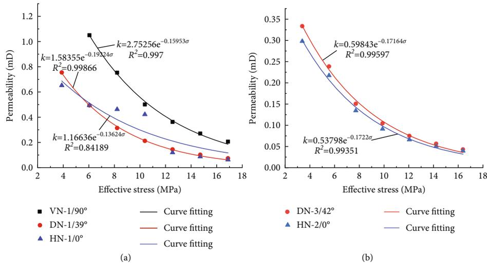
FIGURE 5: Permeability change of different bedding coal samples during stress loading. (a) Gas pressure of 1 MPa. (b) Gas pressure of 2 MPa.
