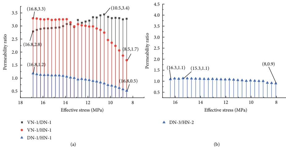
FIGURE 8: Permeability ratios of different bedding coal samples during stress unloading. (a) Gas pressure of 1 MPa. (b) Gas pressure of 2 MPa.
