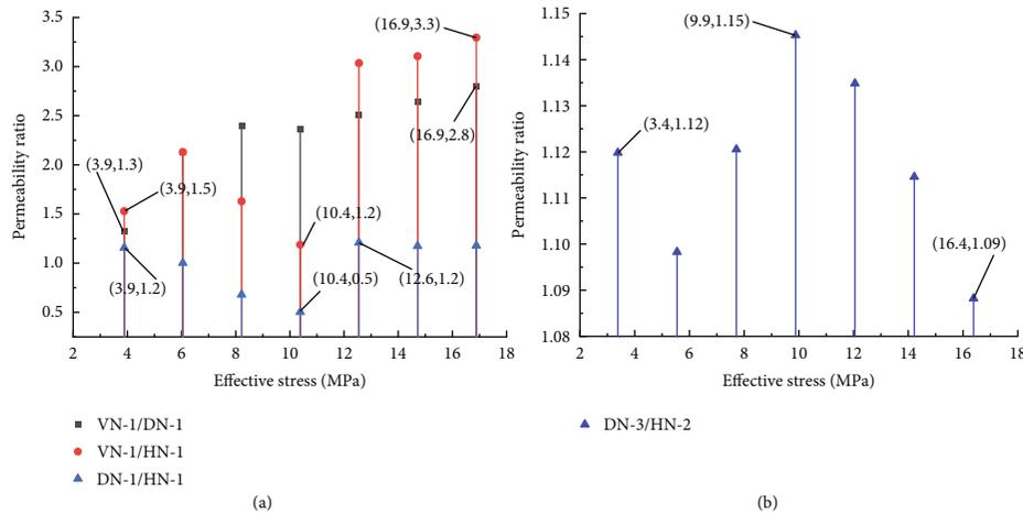
FIGURE 6: Permeability ratios of different bedding coal samples during stress loading. (a) Gas pressure of 1 MPa. (b) Gas pressure of 2 MPa.
