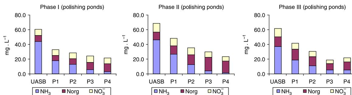
**Figure 3** | Total Nitrogen ( $\text{NH}_3 + \text{Norg} + \text{NO}_3^-$ ) average concentration in the anaerobic reactor and pond effluents over the three operational phases. UASB: anaerobic reactor effluent; Pi: ponds effluents.
