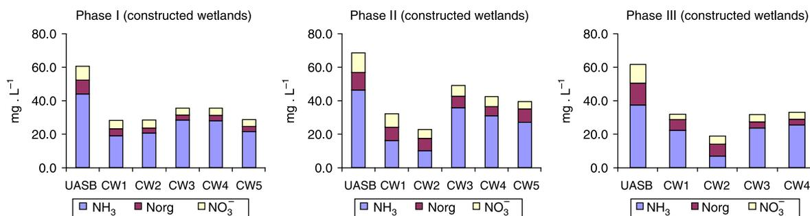
**Figure 4** | Total Nitrogen ( $\text{NH}_3 + \text{Norg} + \text{NO}_3^-$ ) average concentration in the anaerobic reactor constructed wetlands effluents over the three operational phases. UASB: anaerobic reactor effluent; CWi: constructed wetlands effluents.
