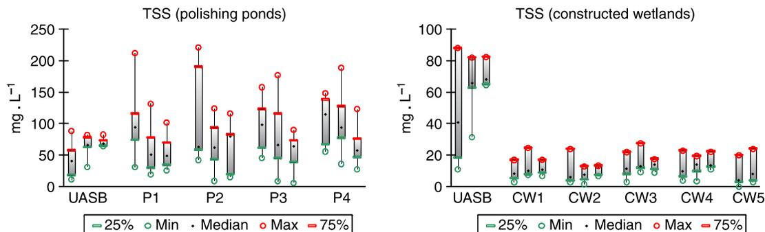
**Figure 2** | TSS concentration in the anaerobic reactor effluent, along the pond series, and in the constructed wetlands effluents over the three operational phases. UASB: anaerobic reactor effluent; Pi: ponds effluents; CWi: constructed wetlands effluents.
