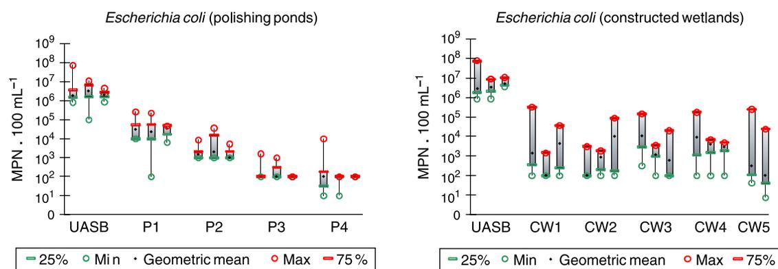
**Figure 5** | *E. coli* concentration in the anaerobic reactor effluent, along the pond series, and in the constructed wetlands effluents over the three operational phases. UASB: anaerobic reactor effluent; Pi: ponds effluents; CWi: constructed wetlands effluents.
