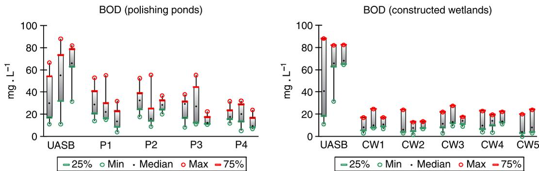
**Figure 1** | BOD concentration in the anaerobic reactor effluent, along the pond series, and in the constructed wetlands effluents over the three operational phases. UASB: anaerobic reactor effluent; Pi: ponds effluents; CWi: constructed wetlands effluents.
