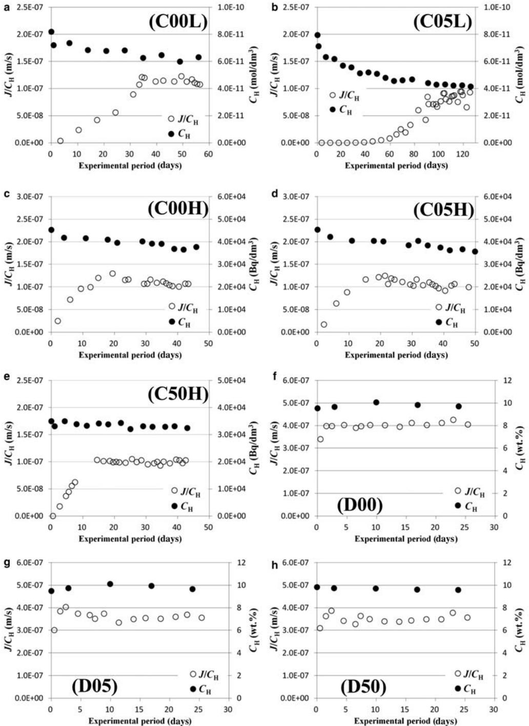
FIG. 2. Changes of flux,  $J/C_H$ , and the tracer concentration in the high-concentration solution,  $C_H$ , with time. <sup>137</sup>Cs was used as the tracer for C00L and C05L (total Cs concentration  $<7 \times 10^{-8}$  mol/dm<sup>3</sup>) and for C00H, C05H and C50H (under saturation with  $1 \times 10^{-4}$  mol/dm<sup>3</sup> non-radioactive Cs), while HDO was used for D00, D05 and D50. All experiments were carried out with  $0.5$  mol/dm<sup>3</sup> NaCl.
