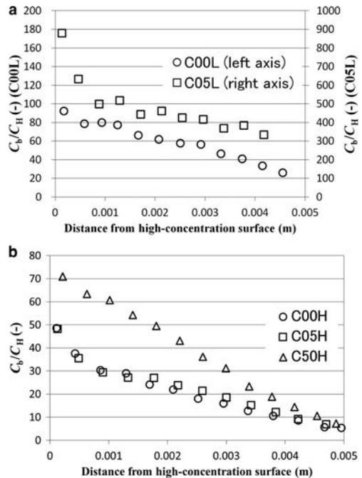
FIG. 4. Concentration profiles of  $^{137}\text{Cs}$  in compacted montmorillonite samples.
