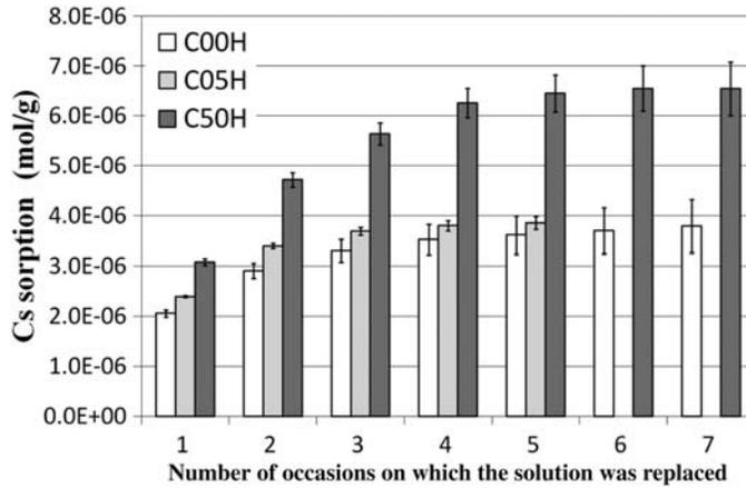
FIG. 3. Amount of Cs sorbed in compacted montmorillonite samples obtained from the saturation procedure with  $0.5 \text{ mol/dm}^3$  of NaCl solution containing  $1 \times 10^{-4} \text{ mol/dm}^3$  non-radioactive CsCl. The error bar indicates  $1\sigma$ .
