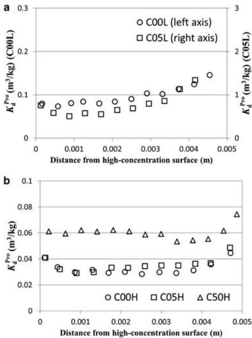
FIG. 5. Profiles of  $K_d^{Pro}$  in compacted montmorillonite samples.
