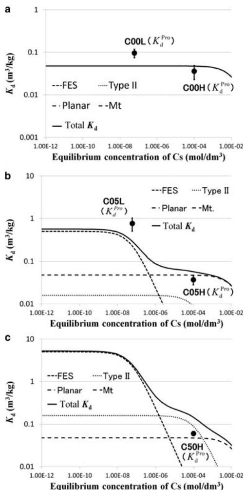
FIG. 6.  $K_d$  values attributed to the sorption at each sorption site and the total  $K_d$  calculated from the models for the samples without illite (a), containing 5% illite (b), and containing 50% illite (c). Mt = montmorillonite.
