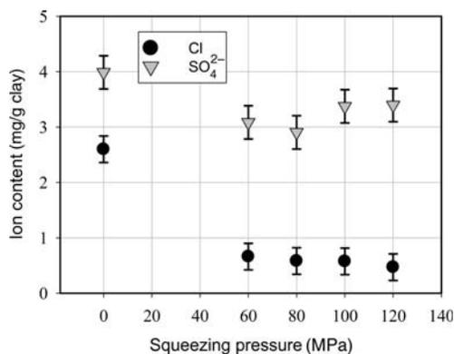
FIG. 8. Chloride and sulfate content as Cl and SO<sub>4</sub><sup>2-</sup>, respectively, in the clay matrix (mg/g of dry clay). The reference sample (0 MPa) is the average of four parallel samples and the error bar is two times the standard deviation for these samples.
