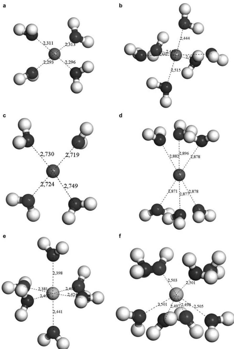
FIG. 3. Cation coordination in montmorillonites based on QM calculations: (a) four-coordinated  $\text{Na}^+$ ; (b) six-coordinated  $\text{Na}^+$ ; (c) four-coordinated  $\text{K}^+$ ; (d) six-coordinated  $\text{K}^+$ ; (e) six-coordinated  $\text{Ca}^{2+}$ ; and (f) eight-coordinated  $\text{Ca}^{2+}$ .
