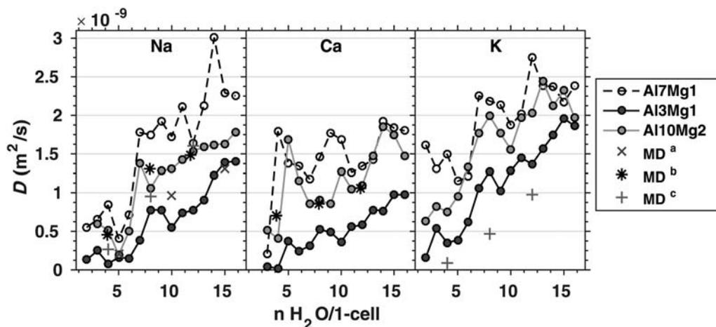
Fig. 11. The 2D interlayer water self-diffusion coefficients (from MD) for Na-, Ca- and K-montmorillonites and the MD results from: (a) Holmboe & Bourg (2014); (b) Greathouse *et al.* (2015); and (c) Boek (2014) (given in 3D).
