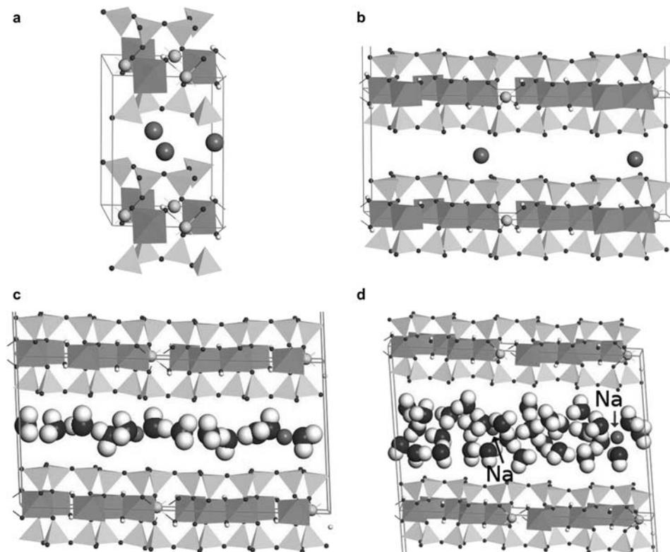
FIG. 2. (a) The unit cell of Na-montmorillonite from QM calculations; (b) the model structure ( $1 \times 3 \times 1$  unit cells) for MD simulations, and Na-montmorillonite with (c) four and (d) ten water molecules per unit cell. Tetrahedral sheet: Si. Octahedral sheet: Al. Spheres in octahedral sheet: Mg. Small spheres in the octahedral and tetrahedral sheets: O. Interlayer: Na and water.
