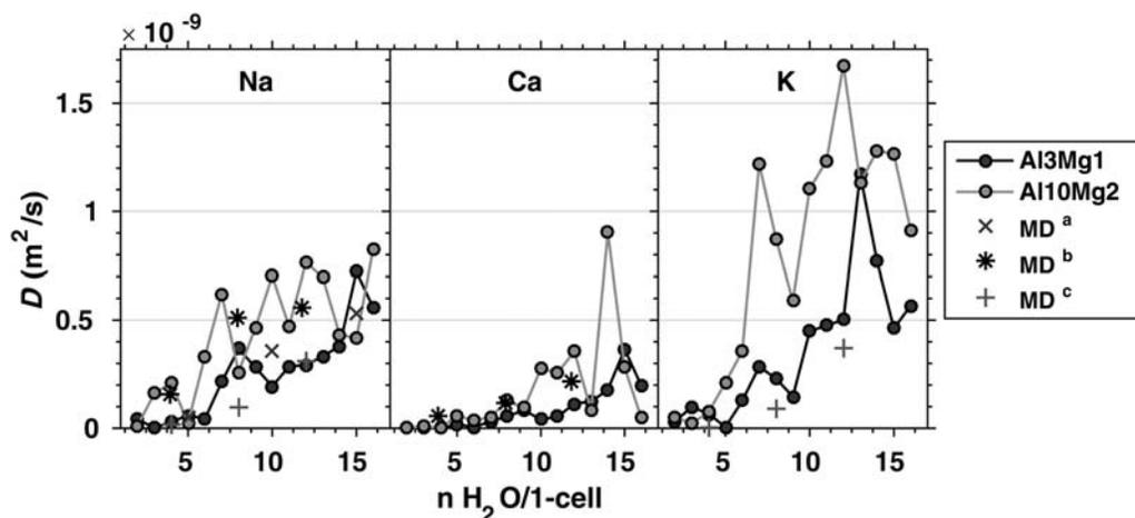
Fig. 12. The 2D interlayer cation self-diffusion coefficients (from MD) for Na-, Ca- and K-montmorillonites and the MD results from: (a) Holmboe & Bourg (2014); (b) Greathouse *et al.* (2015); and (c) Boek (2014) (given in 3D).
