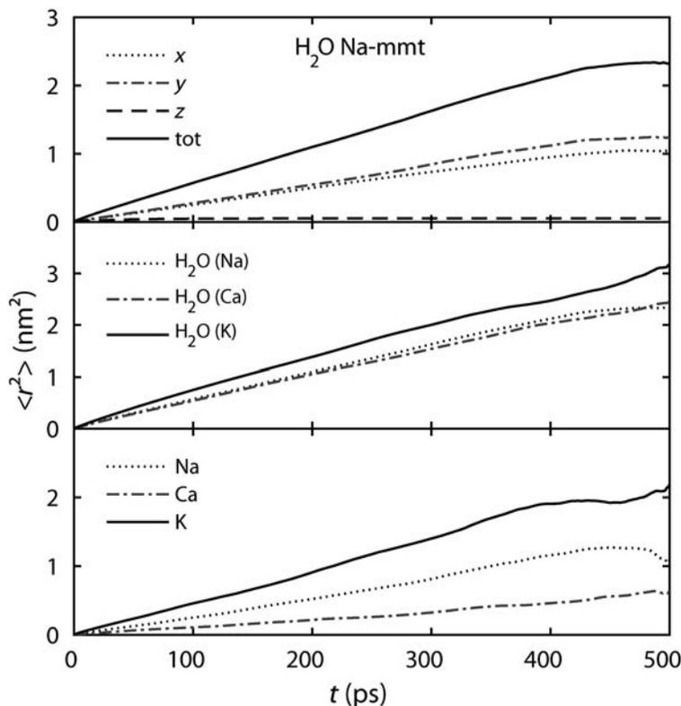
FIG. 10. MSD from MD calculations:  $x$ ,  $y$ ,  $z$  and total components for interlayer water in Na-montmorillonite with 10  $\text{H}_2\text{O}$ /unit cell (top), interlayer water (O) in Na-, Ca and K-montmorillonites with 10  $\text{H}_2\text{O}$ /unit cell (middle) and the interlayer cations (bottom).
