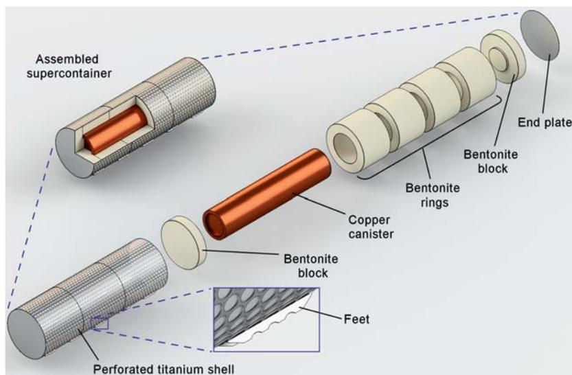
FIG. 1. Illustration of the emplaced components in the KBS-3H disposal concept (based on Posiva, 2012). Exploded assembly drawing showing a supercontainer with copper canister, bentonite buffer and perforated Ti shell.
