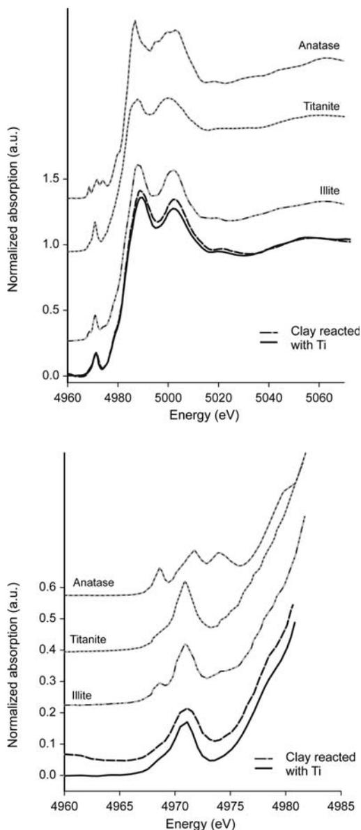
FIG. 11. XANES spectra (Ti pre-edge structure) of synthetic montmorillonite samples reacted with Ti released from corroding Ti foils. Reaction periods were 218 (solid line) and 601 (dashed line) days at 80°C and neutral pH. For comparison additional spectra of reference materials are shown; upper: XANES spectra; lower: close-up of pre-edge spectral region.
