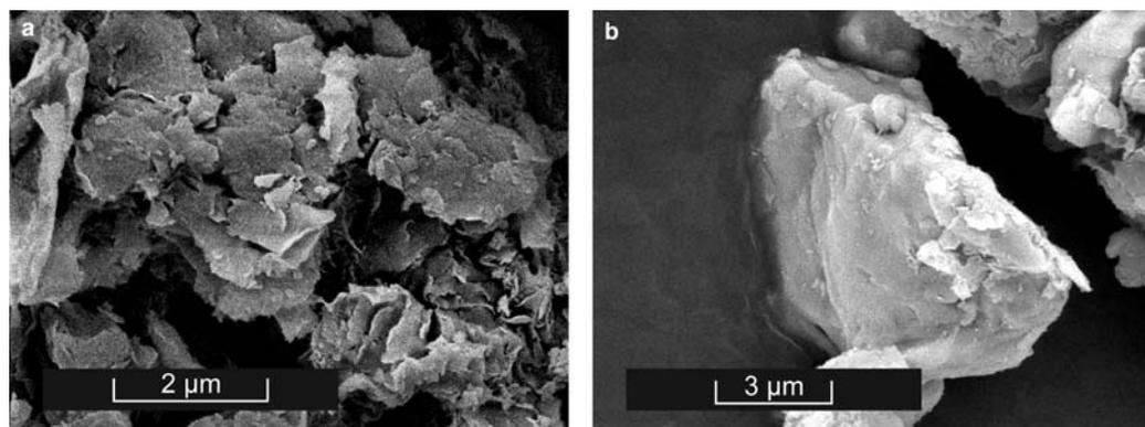
FIG. 6. SEM image of synthetic Na-montmorillonite: (a) reacted for 1 month in neutral conditions in the presence of Ti powder; (b) SEM image of a  $\mu\text{m}$ -sized Ti particle partially covered by clay platelets.
