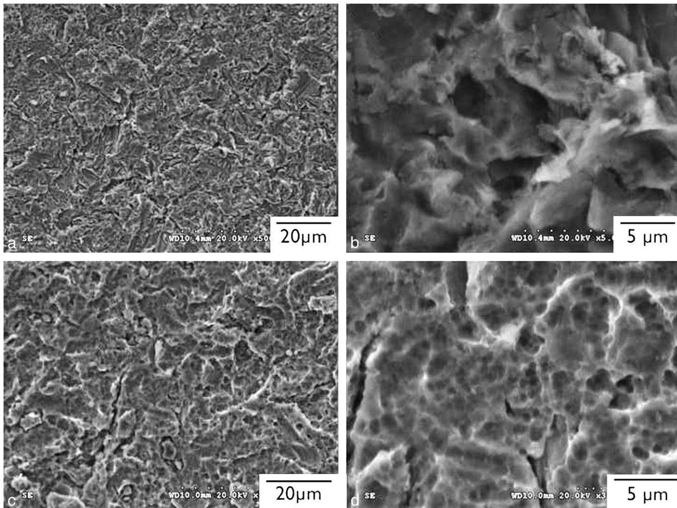
**FIGURE 1.** Scanning electron microscopy micrographs show morphology of (a) resorbable blasting media experimental and (c) alumina-blasted/acid-etched control surfaces. Higher magnification of the respective surfaces (b and d) did not reveal evidence of particle embedding in either surface.
