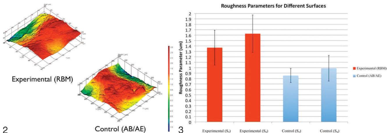
**FIGURES 2 AND 3.** **FIGURE 2.** Micrometer length scale optical interferometry reconstructions showing higher  $S_a$  and  $S_q$  values for the resorbable blasting media compared with the control surfaces. **FIGURE 3.** Statistical summary (mean  $\pm$  95% CI) of surface roughness parameters at the micrometer level length scale. Statistical  $P$  values for the experimental  $S_a$  and  $S_q$  were significantly higher compared with control groups ( $P < .05$ ).
