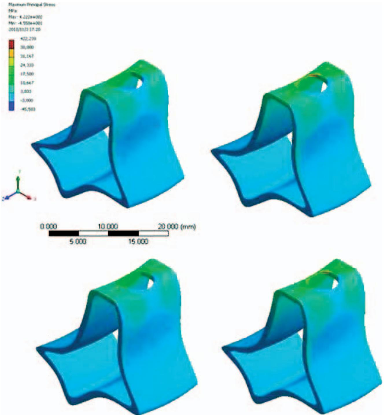
**FIGURE 4.** Maximum principal stress on cortical bone in models RS (regular platform and straight abutment), RA (regular platform and angulated abutment), SS (platform switching and straight abutment), and SA (platform switching and angulated abutment).
