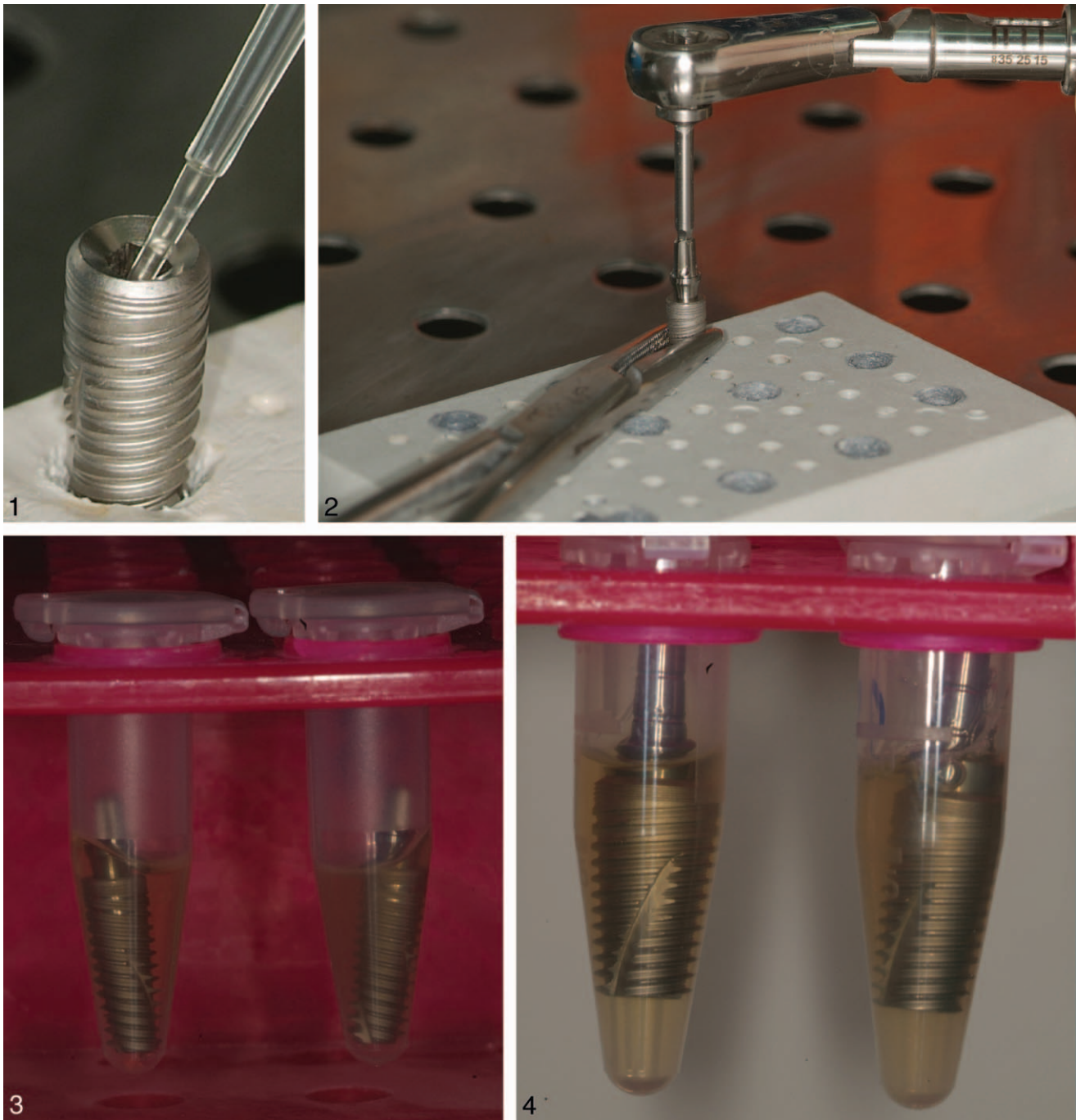
FIGURES 1–4. FIGURE 1. The inner part of implants inoculation with a viable bacteria suspension. FIGURE 2. An assembled implant-abutment with an implant torque controller. FIGURE 3. Cone Morse implants placed into nutrient solution. Left: no contamination. Right: turbidity of the broth as sign of bacterial penetration. FIGURE 4. The internal hexagon implants placed into nutrient solution. Left: no contamination. Right: turbidity of the broth as sign of bacterial penetration.
