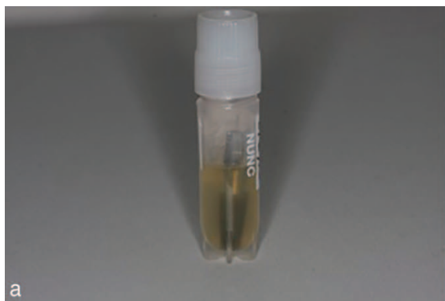
FIGURE 2. (a) Implant and abutment of Group 1 in a plastic container with the bacterial solution. (b) Implant and abutment of Group 2 in a bacterial solution subjected to dynamic loading.
