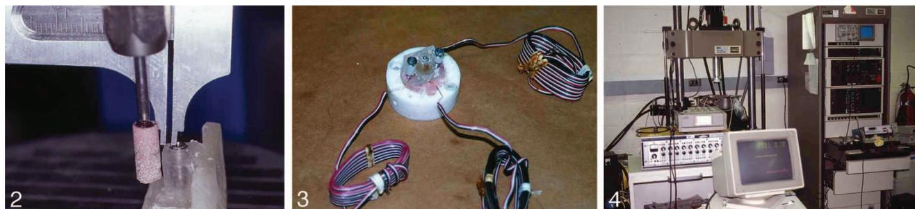
**FIGURE 2–4.** **FIGURE 2.** An experimental sample prior to placing the strain gages. The walls of the resin cylinder containing the implant are being reduced to a thickness of 1 mm. **FIGURE 3.** A completed specimen with the strain gages attached. The implant is in the center of the sample. The leads from the strain gages attached to the acrylic extend outward from the sample. **FIGURE 4.** The MTS system with loaded sample.
