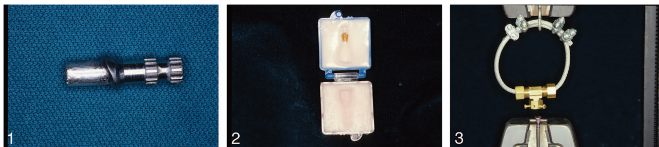
FIGURES 1–3. FIGURE 1. 0.001-inch thickness platinum foil was adapted onto the abutment surface as a die spacer. FIGURE 2. Split mold technique used to wax up implant superstructures. FIGURE 3. The testing jig with 3 side screws was attached to the universal testing machine to test the cement failure load.
