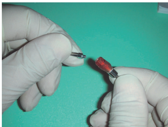
FIGURE 2. Image of the new appliance fabricated for measuring the tightening forces.
