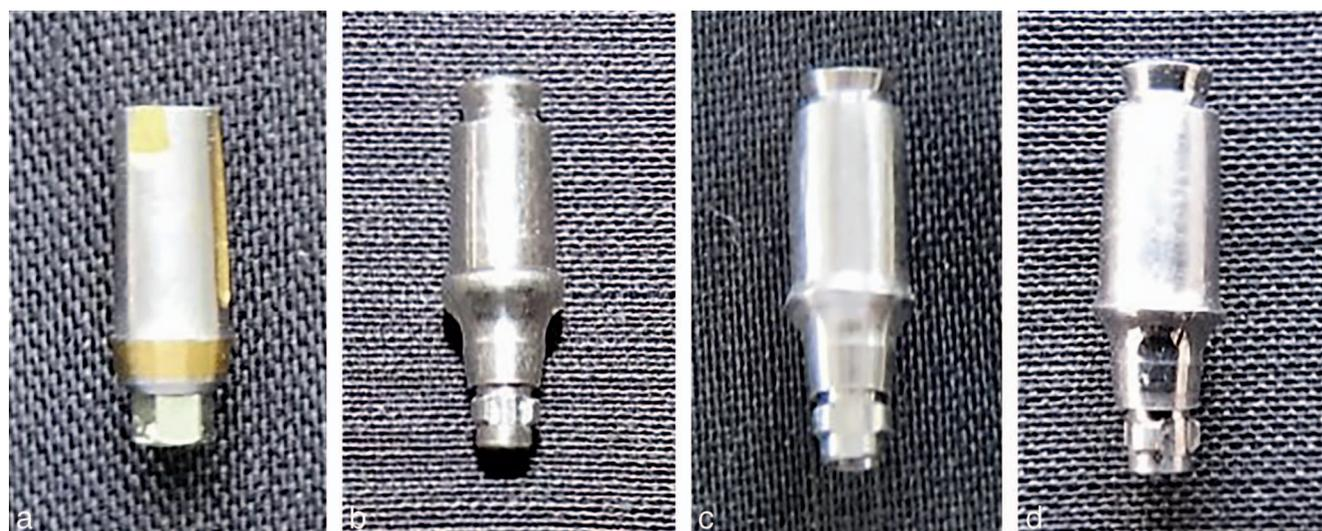
**FIGURE 3.** (a) Standard abutments (Control Group). (b) Myriad Plus abutments as supplied by the manufacturer (Group 1). (c) Myriad Plus abutments milled to a depth of 1 mm (Group 2). (d) Myriad Plus abutments milled to a depth of 1.5 mm (Group 3).
