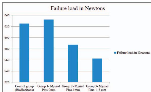
**FIGURE 5.** Mean failure loads of the various groups.
