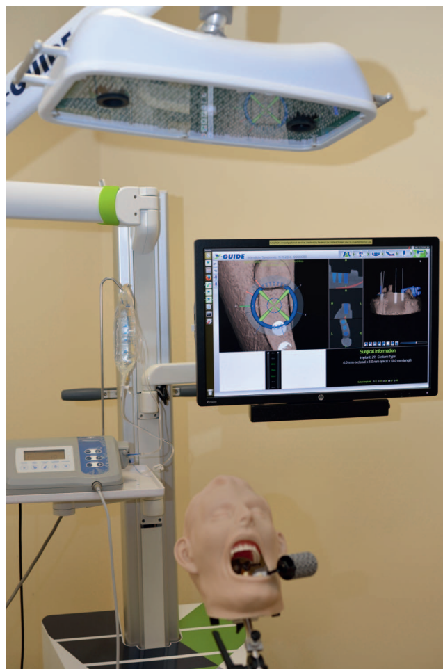
FIGURE 3. Simulated surgical situation showing manikin, Sawbones model, and patient-tracking array with X-Guide above.
