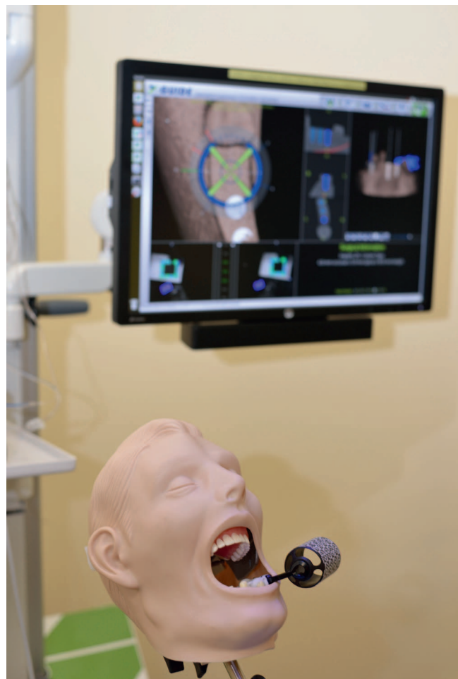
FIGURE 1. X-Clip holding the patient-tracking array on Sawbones model.
